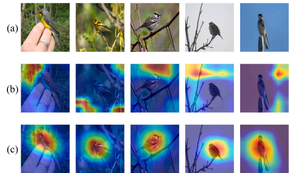
Fig. 3. Visualization with GradCAM on CUB200, where (a) raw images of new classes, (b) results without using our proposed pseudo incremental relation complementation learning scheme, (c) results with using our proposed pseudo incremental relation complementation learning scheme.
